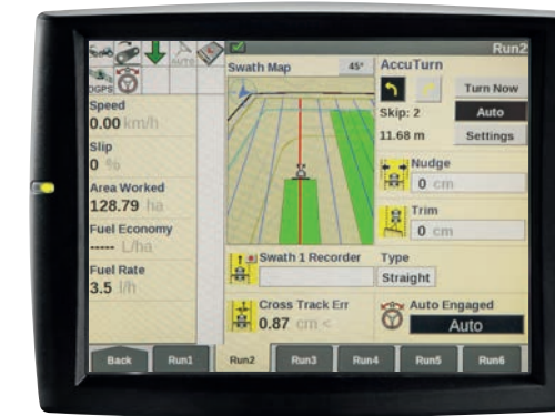
Automated turning process with AFS AccuTurn Pro
